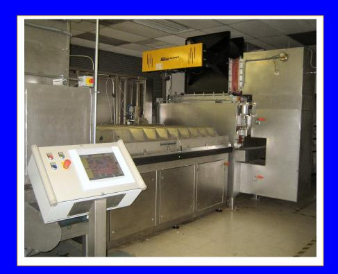
The GLS works for safety, hurricane, ballistic, fire- rated and other laminated glass products. It can also be used to encapsulate different kinds of solar modules, including those with backsheets. It is suitable for clear, coated, mirrored or colored glass in an annealed or tempered state and for laminating products sensitive to pressure and temperature, as well as products with decorative and functional inserts.
