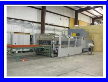
The entire laminating process can be accomplished in the vacuum laminator where trapped air, moisture, and gases are completely pumped off while the sandwich is being heated. The sandwich lays freely on the conveyor without being subjected to pressure.
